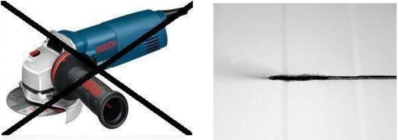
Fig. 2. Inappropriate tool for cutting panels.
